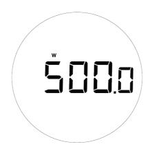
Indicated by a W in the top left corner of the display. The weighing mode is Orion's smart scale mode. It will function like an industrial weighing scale. To switch to weighing mode, long press the **Power** button and rotate the dial until it display [SCALE], then press **Power** button to confirm.
