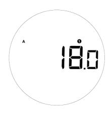
There will be an 'A' indicator on the top left corner of the display when in automatic dosing mode. The auto dosing mode is designed to dose automatically whenever a container is placed on the Orion platform. When the display shows 'Ready,' it means the Orion is in auto dosing mode and any container placed on top of the platform will automatically dose to the target weight.
